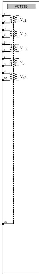
Module no. 33 (VT x 5) Only for 1/3 rack
